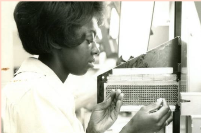
Women employees of Raytheon assembled core memory for the Apollo Guidance Computer by threading metal wires through rings. (This unnamed woman was described as a "space age needleworker" in a Raytheon press kit.) Courtesy of the collection of David Meerman Scott, Raytheon public relations
