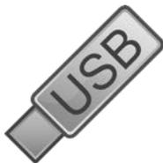
USB Flash storage devices are small printed circuit boards that communicate with computers. Capacity can be up to 1 TB (terabyte) as technology improves. Data can last up to 10 years & up to 100,000 write/erase cycles depending on the use. Cheaply made, it will last between two and four years. Always make a stable copy of your most precious data on another drive rarely used.
